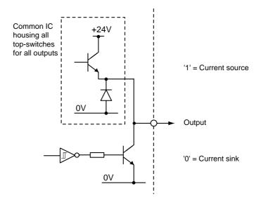
Figure 3-15. User Output Circuit
